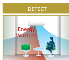
Only one person in the room. Detects wasted cooling area.
